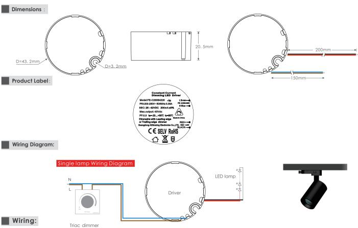
The output wire: 20AWG red and black PVC cable ,length 200-230mm,wire stripping requirement:5-7mm
